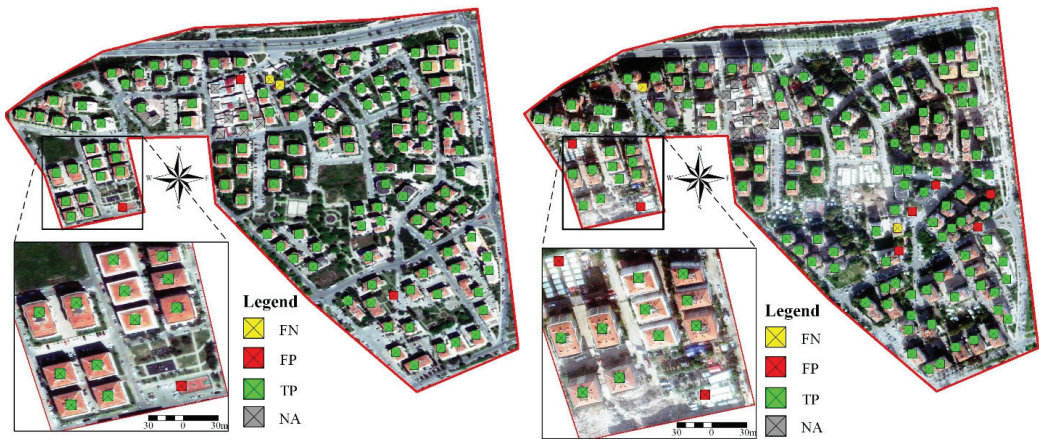
Figure 9. Pre (left) and post (right) earthquake building detection from Maxar satellite imagery.
