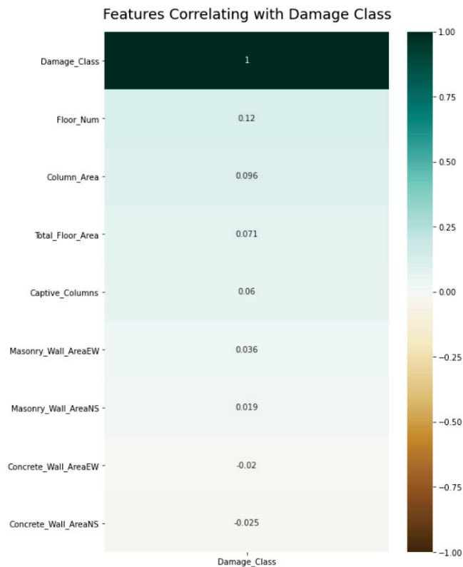
Figure 9. Heatmap illustrating correlation coefficient between independent and dependent variables.
