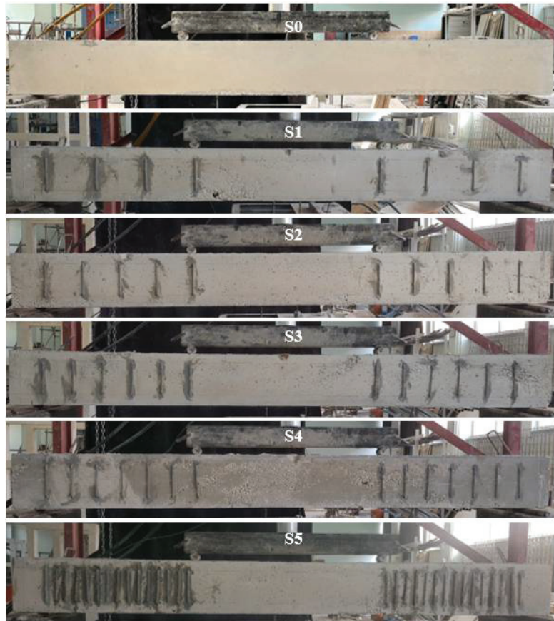
Figure 5. Pre-experiment view of reference and reinforced beams.
