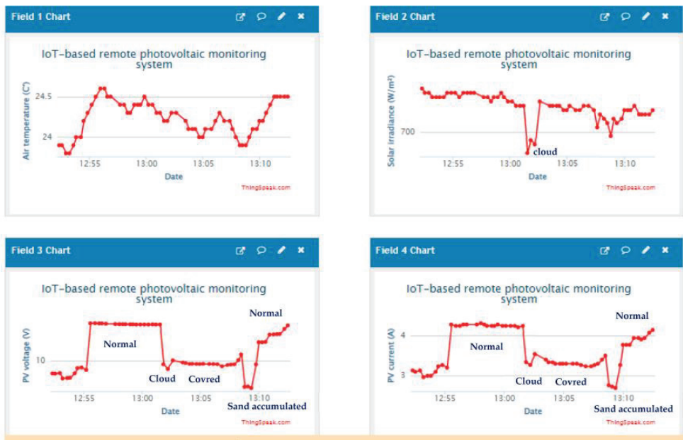
Figure 12. Monitored data (air temperature, solar irradiance, DC voltage, and DC current) based on ThingSpeak application.
