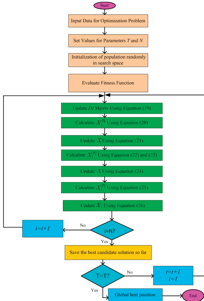
Figure 4. The flowchart for the suggested DTBO approach.
