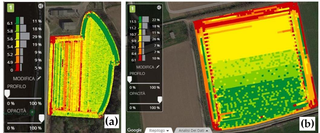
**Figure 1.** The forward speed of two different sowing operations on soil with different skeleton levels. (a) reports operation on soil with high skeleton which allowed a maximum speed of 5.6 km h<sup>-1</sup>. (b) reports the same tractor and seeder on soil without skeleton correctly sowing at 11.5 km h<sup>-1</sup>.
