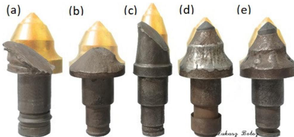
**Figure 1.** Worn conical picks [14]: (a,c) asymmetrical forms; (b,d,e) symmetrical forms.
