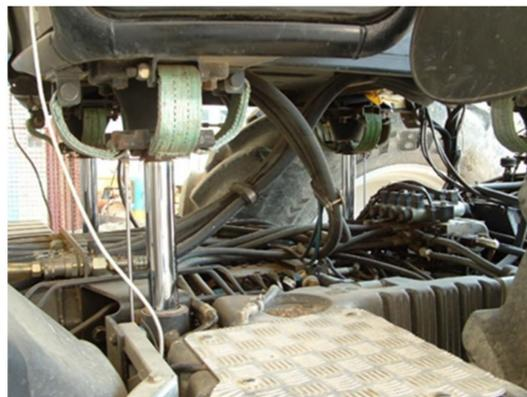
**Figure 2.** Particulars of a hydraulic cylinder and of the silent block on its top.
