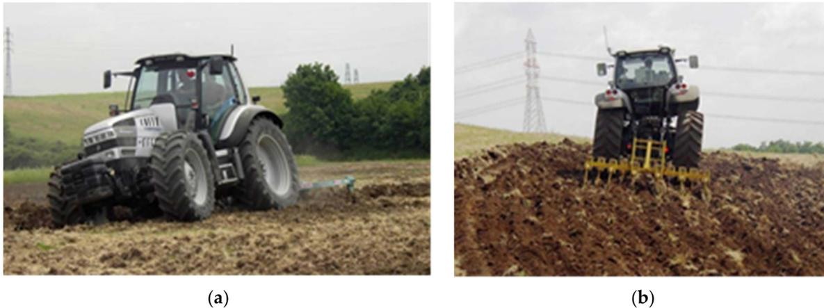
**Figure 5.** The tractor equipped with the self-levelling cab during the tests with the plough (a) and the subsoiling plough (b).
