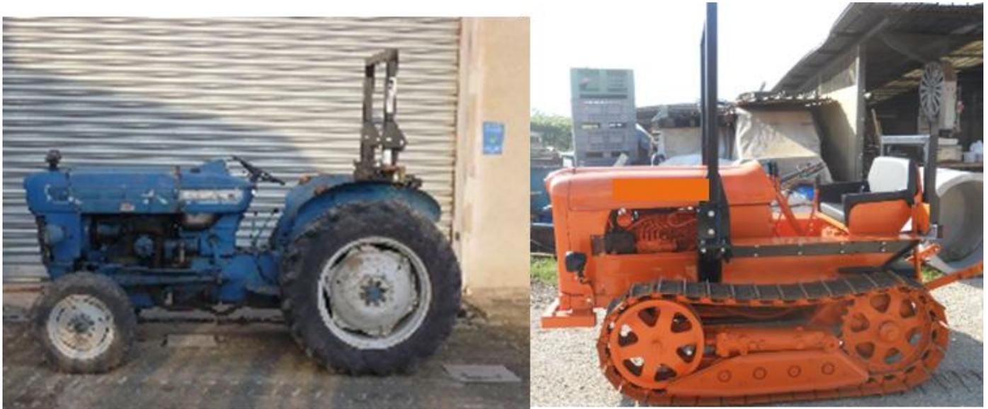
**Figure 1.** Examples of a rear-mounted FROPS (left) and a front-mounted FROPS (right).
