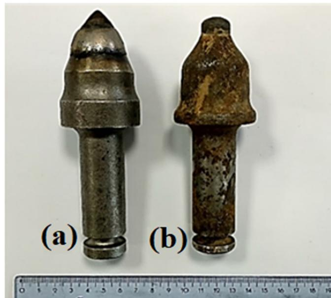
**Figure 5.** Destruction of the working tool: (a) new tool; (b) worn tool.
