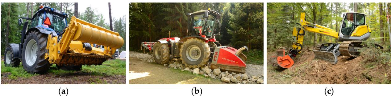
**Figure 4.** Machines for the creation, modification and reconstruction of forest roads: (a) for UKT; (b) for special machines; (c) for hydraulic manipulators.
