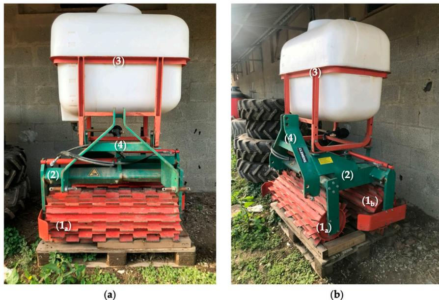
**Figure 3.** Front (a) and lateral (b) view of the commercial roller crimper Clemens Eco-Roll type: (1<sub>a,b</sub>) roller crimpers; (2) hexagon frame; (3) tank; (4) three-point hitch.
