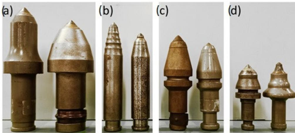
**Figure 3.** Often used types of conical picks: (a) for coals and rocks; (b) for salts; (c) for road, rocks, concrete; (d) for roads, concrete and asphalt.
