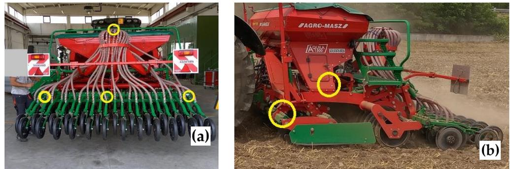
**Figure 12.** (a): the position of the triaxial accelerometers 1, 2 and 3 (on sowing elements, yellow circles) and the position of the microphone in the middle of the ladder railing of the upper portion on the hopper (yellow circle). (b): the position of the triaxial accelerometers 4 and 5 (yellow circles).
