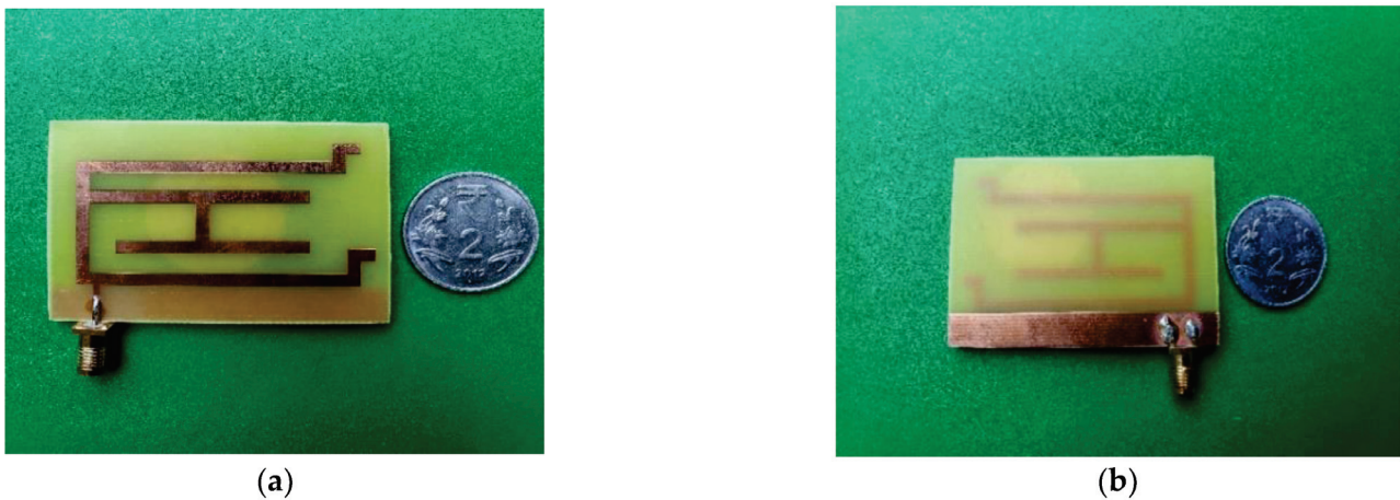
Figure 3. Fabricated monopole antenna. (a) Top view (b) Back view.
