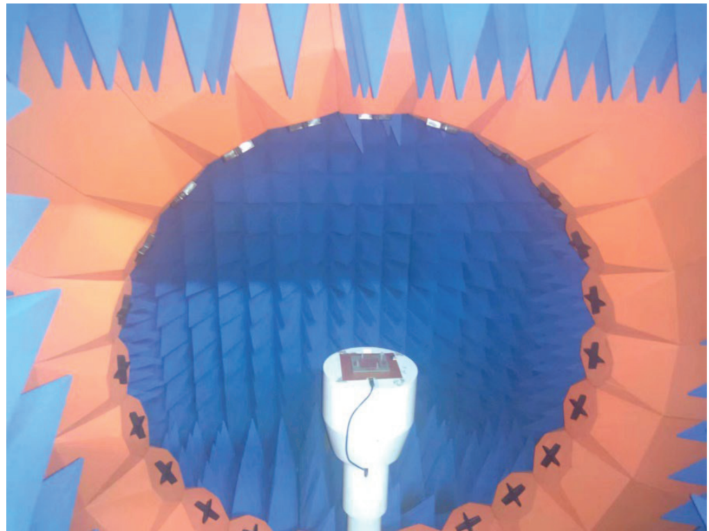
Figure 7. Antenna prototype testing scenario in the chamber.
