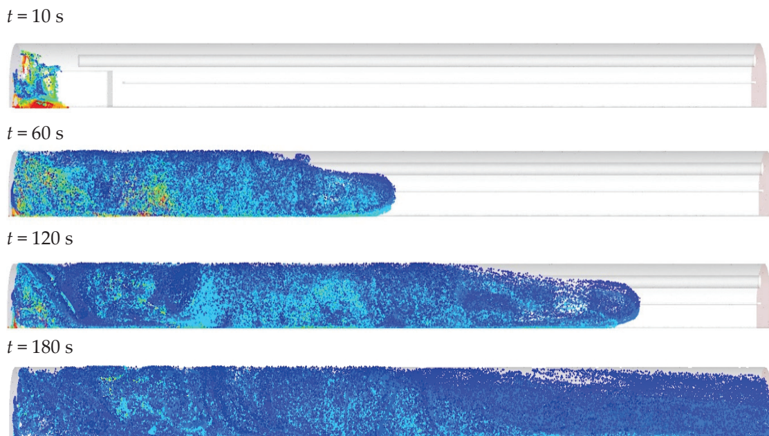
Figure 5. Distribution of different-sized dust particles in the dog heading at various time points for total dust rate = 0.00125 kg/s.
