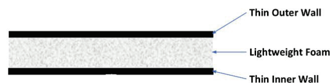
Figure 1. Sketch of a Dual-Wall Configuration Stuffed with Light-weight Foam.
