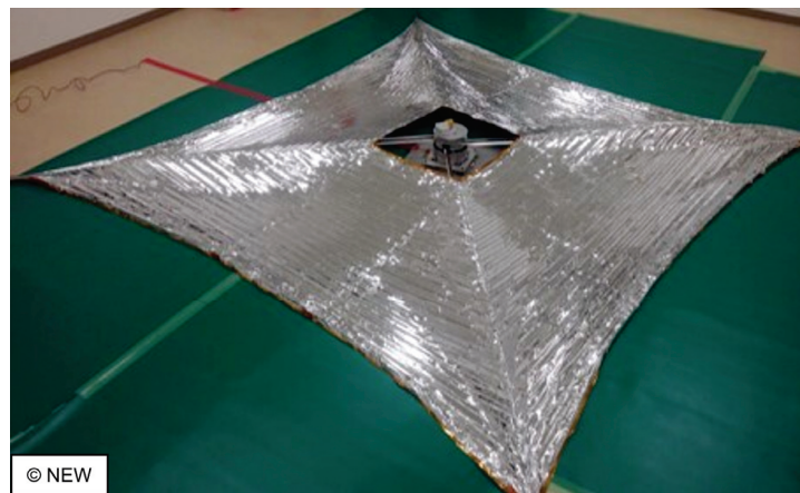
Figure 2. Deployed configuration of DOM: De-Orbit Mechanism.
