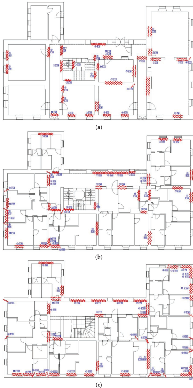
Figure 7. Damage patterns (red marks): (a) ground floor, (b) first floor, and (c) second floor.
