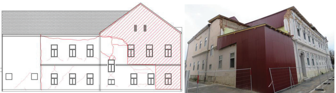
Figure 11. Northwestern façade plan with marked damage.
