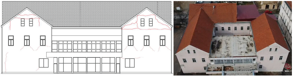
Figure 12. Northeastern façade plan with marked damage.
