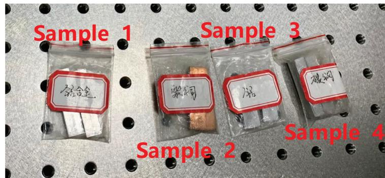
**Figure 6.** Test samples, sample 1 (aluminum alloy), sample 2 (copper), sample 3 (pure aluminum), sample 4 (carbon steel).
