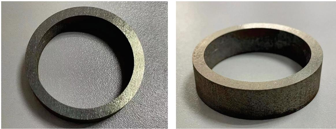
**Figure 16.** Ring test specimen machined by WEDM.
