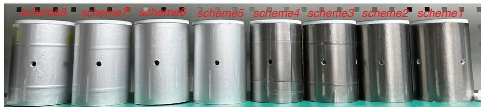
**Figure 2.** Amorphous and nanocrystalline inner magnetic shield layers.
