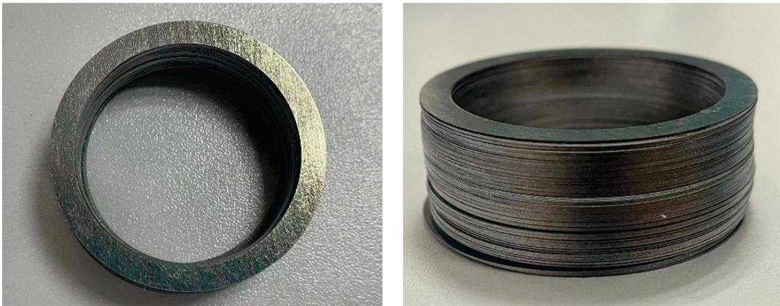
Figure 17. Laser cutting shaped ring test specimen.
