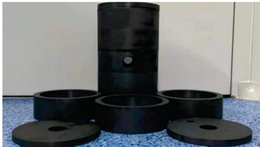
**Figure 4.** Ferrite magnetic shield and magnetic annulus. The ferrite magnetic shield has four through holes with a diameter of 25 mm in the transverse direction and two through holes with a diameter of 35 mm in the longitudinal direction.
