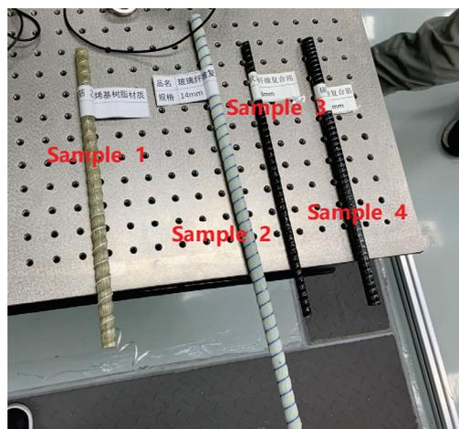
**Figure 5.** Test samples, sample 1 (vinyl resin), sample 2 (glass fiber), sample 3 (basalt fiber composite bar), sample 4 (carbon fiber composite bar).
