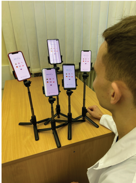
Figure 2. The experimental setup of five different smartphone devices modeled in this study (iPhone SE, iPhone PRO MAX 13, Huawei P50 pro, Samsung S22 Ultra, and OnePlus 9 PRO).
