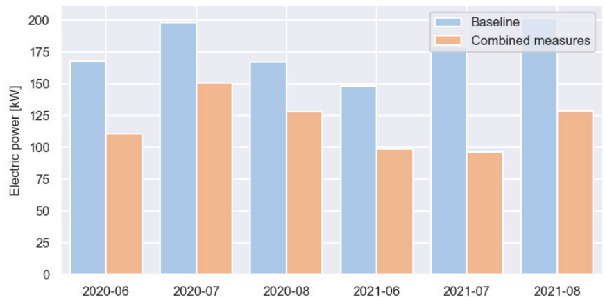
Figure 18. Average chilled water system electric power per month for the baseline and the combined measures during summer 2020 and 2021.
