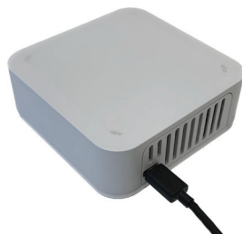
Figure 3. Custom-built IAP sensor node (Own representation).
