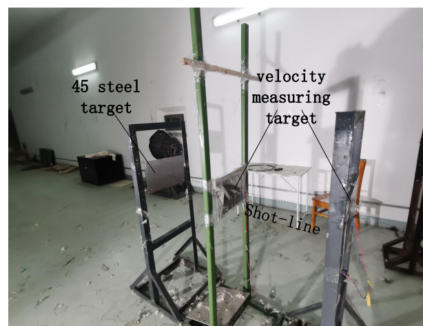
Figure 3. The set-up of the ballistic gun test.
