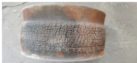
Figure 2. Roller wheel after high temperature failure (SUS304).
