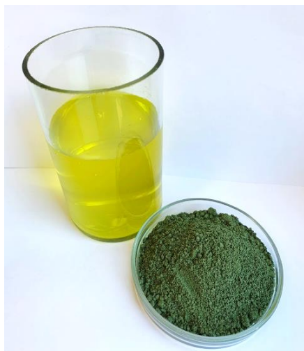
Figure 1. Liquid and solid phases of catalyst slurry.
