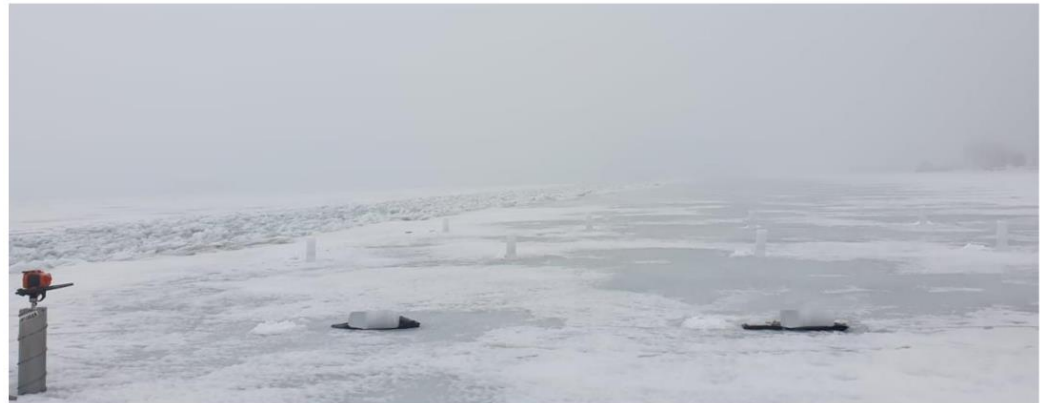
Figure 3. The study location for the investigation level ice was adjacent to the test channel (TCh01 27 March 2021), where cores were examined from a test grid, starting approximately 5 m from the channel edge, and extending up to 30 m towards the shoreline. Cores were also collected along the channel direction for a distance of 30 m. The spacing between cores was 5 m.
