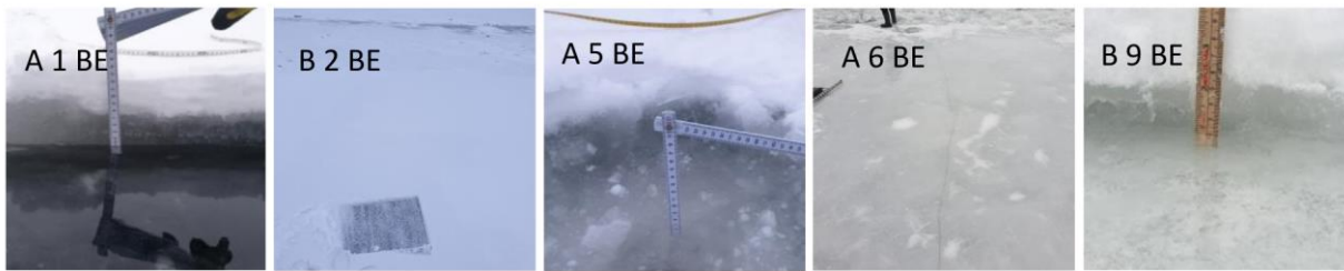
Figure 6. The level ice in the vicinity and adjacent to the channel (TCh02) was flooded after the ship passages. A 1 BE shows the adjacent level ice flooded instantly after the first ship passage, whereas B 2 BE shows the level ice before the second ship passage, with the slush frozen to snow ice.
