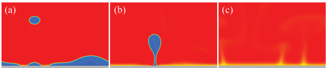
Figure 3. The density contour plots illustrating the boiling process at low surface superheat, \Delta T = 0.045 T_c . (a) lyophobic surface ( \theta = 116^\circ ), (b) neutral surface ( \theta = 90^\circ ) (c) lyophilic surface ( \theta = 38^\circ ).
