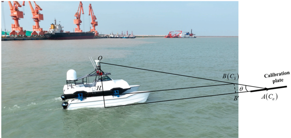
Figure 4. Camera height and pitch angle model.
