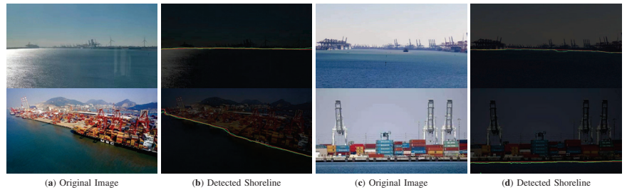
Figure 8. The results of our method on the port dataset for shoreline detection. The green line is the detected shoreline, the red line is the reference shoreline, and the yellow portion represents the overlap between the two.
