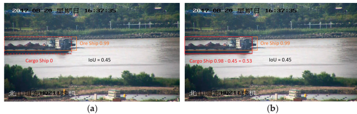
Figure 4. Processing results of overlapping targets by NMS and Soft-NMS; (a) NMS processing mode; (b) Soft-NMS processing mode.
