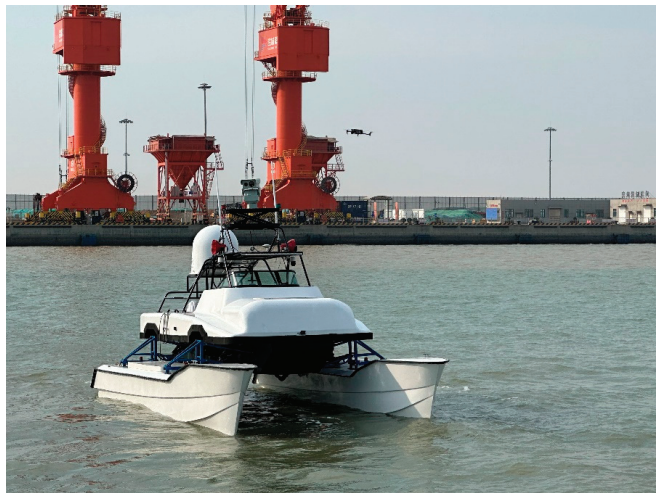
Figure 6. Cooperative USV-UAV platform.
