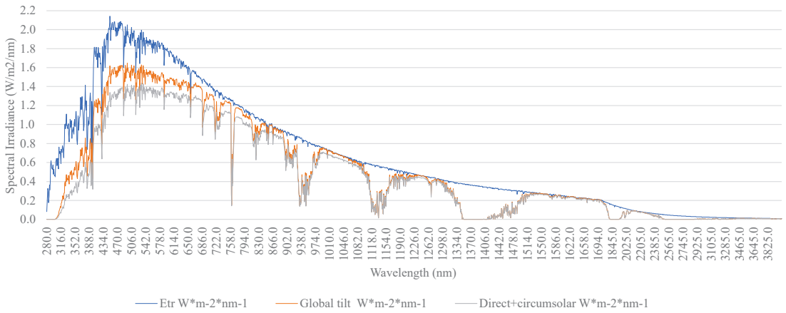
Figure 2. ASTM G-173-03 standard graphic on site, including the extraterrestrial irradiance (solar spectrum at top of atmosphere), global tilted irradiance, and direct (+ circumsolar) irradiance.
