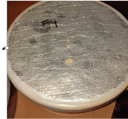
Figure 4. Mould growth on specimen E.
