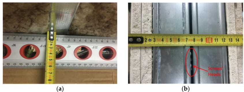
Figure 4. Geometry details of the measured double pane LSF wall test sample. (a) Expansible MW around steel stud; (b) Steel track distance.
