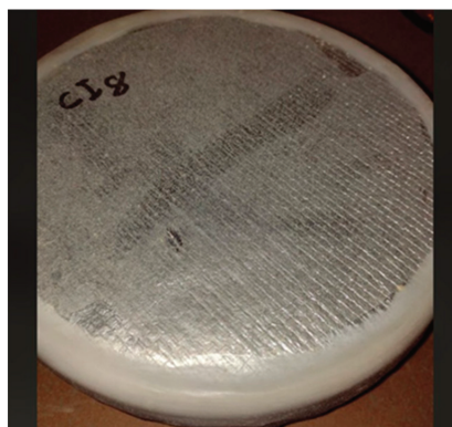
Figure 3. Mould formation on specimen D.
