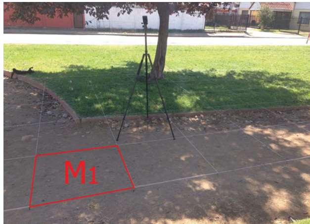
Figure 4. Location of the spectrometer in a quadrant to take the measurements.
