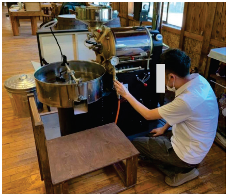
Figure 4. A roaster adjusting the heating power based on the analogue thermometer.
