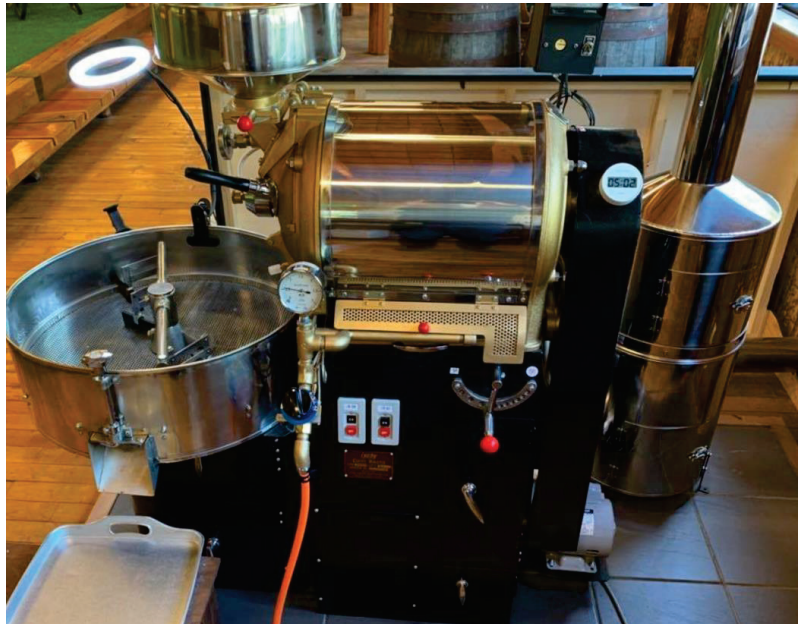
Figure 3. Small commercial roaster with a capacity of 4 kg.
