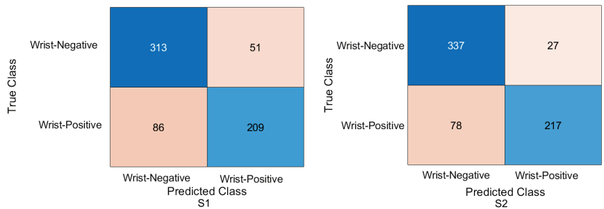
Figure 10. Confusion matrix of the Xception model on the test set with two different training scenarios of the wrist task.
