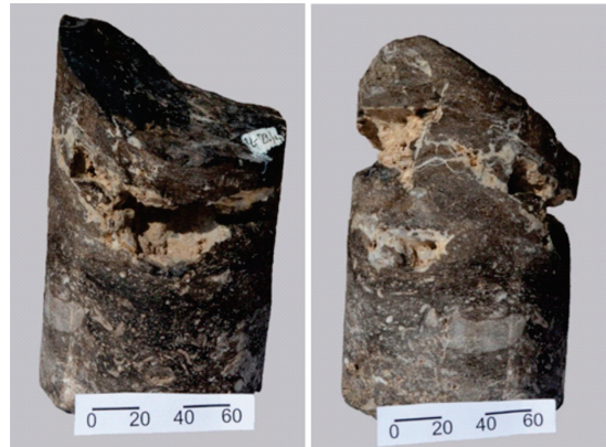
Figure 5. Inclined joint of tectonic separation in Famennian–Carboniferous rocks (detail of Figure 4(3)) with subsequent development of vugginess and new formations of carbonate minerals.
