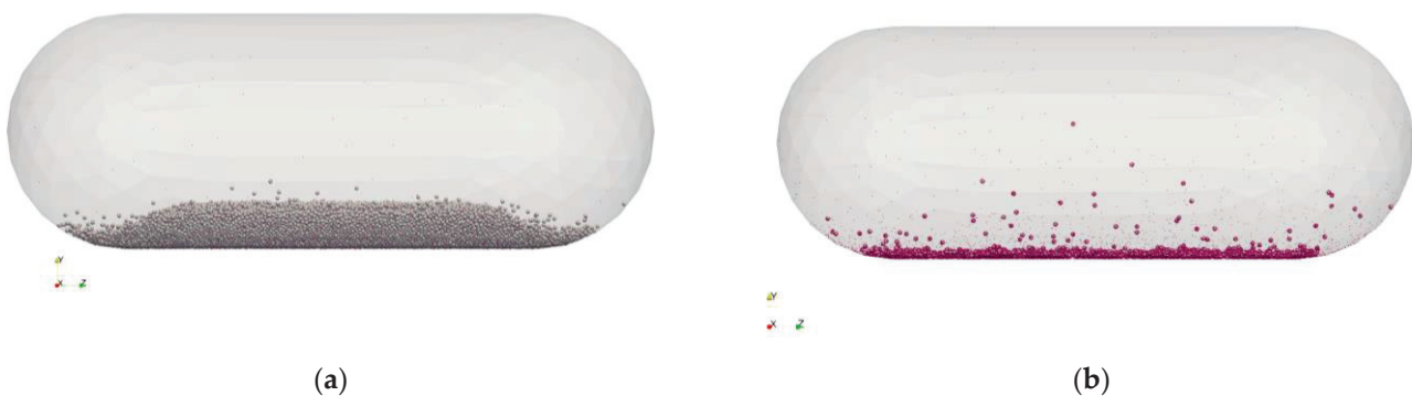
Figure 5. Powder configuration after gravity settling: (a) 25 mg (after 40 ms) and (b) 1 mg (after 200 ms). Carrier particles are shown in gray, and API particles are in purple.
