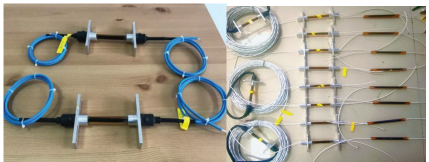
Figure 4. The self-developed I-shaped strain sensor made by encapsulated cylindrical MWCNT/EP composite.
