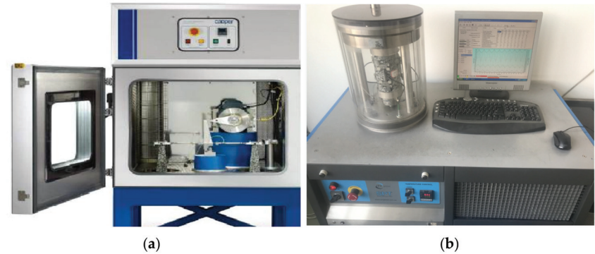
Figure 1. Schematic diagram of 2PT (a) and SPT (b) loading equipment.
