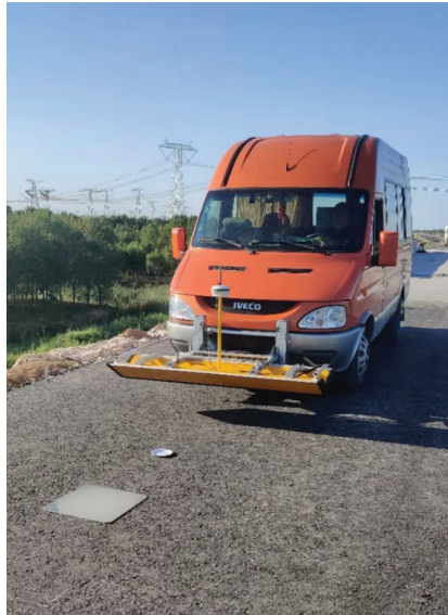
Figure 1. Three-dimensional ground-penetrating radar (GPR) inspection vehicle.
