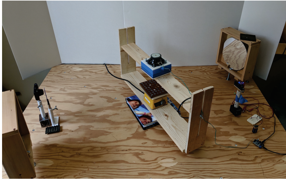
Figure 2. Schematic drawing and photograph of the experimental Schlieren configuration.
