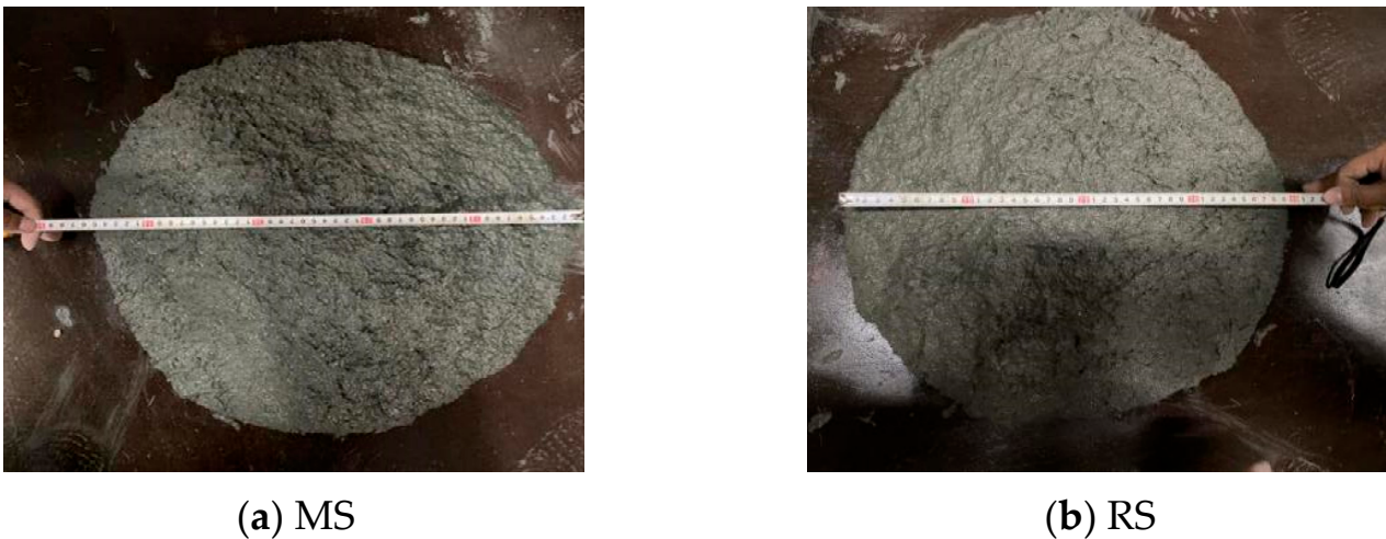
Figure 2. Concrete slump spread test.
