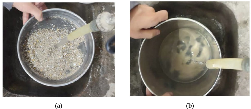
Figure 1. Ceramic mold shells washing process: (a) Washing of the particles with dimensions between 0.125 mm and 4 mm; (b) Washing of the particles with dimensions lower than 0.125 mm.
