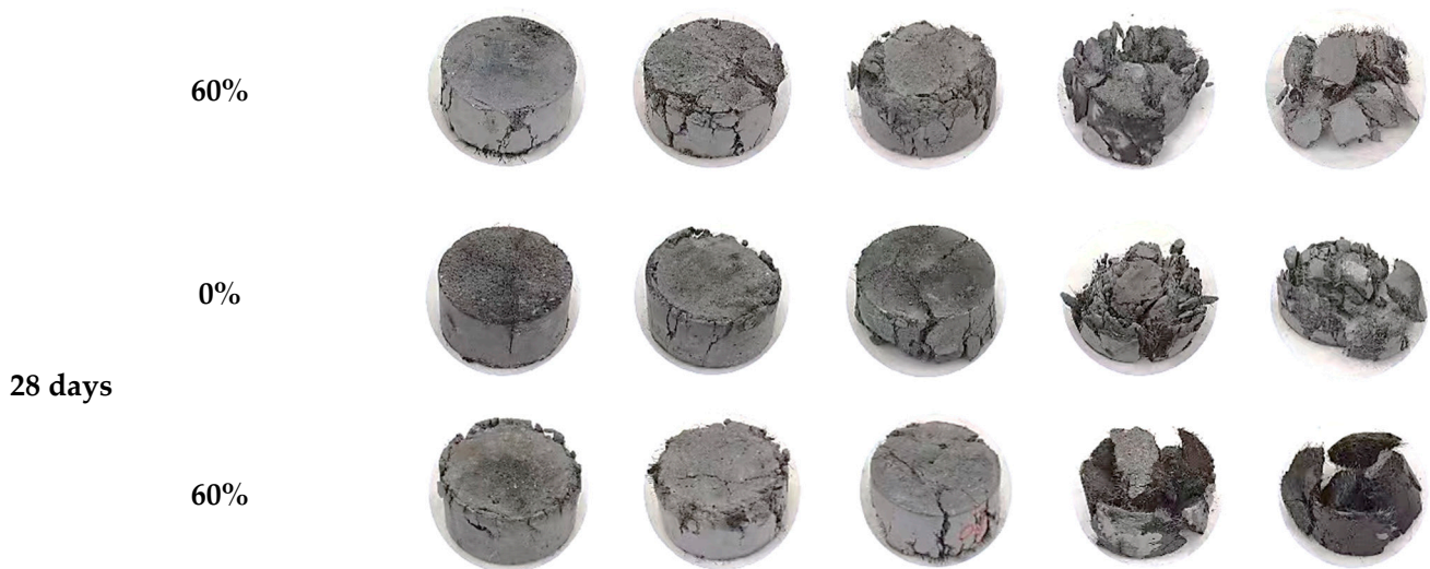
Figure 14. Typical failure modes of HSFRC specimens under dynamic compression tests.
