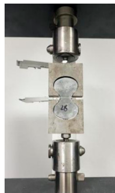
Figure 4. Steel fiber pullout test.
