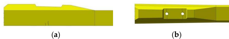
Figure 1. Transverse crack in a rail seat section: (a) lower part crack in the rail seat section; (b) upper part crack in the rail seat section.
