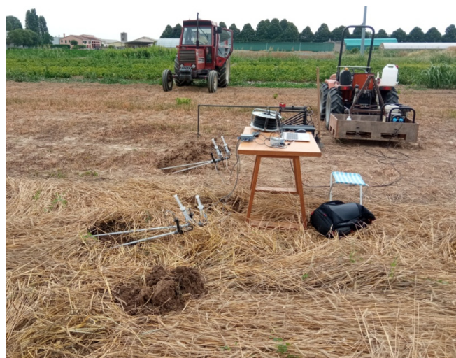
Figure 5. Installation position of the Bolling probe to measure the mean normal stress with different cover crop mulch treatments.
