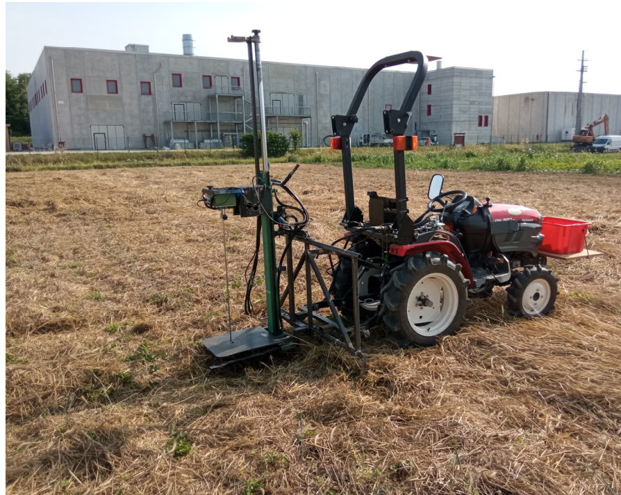
Figure 4. A penetrometer was installed on an iron frame with hydraulic ram to insert the cone tip at constant speed in the soil.
