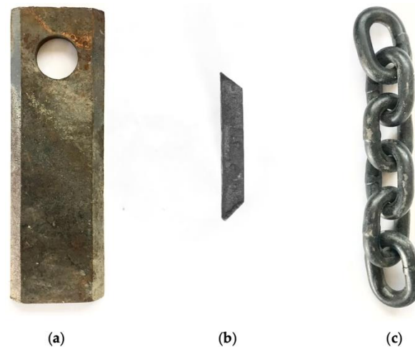
Figure 2. Different kinds of cutting tool: (a) blade; (b) cross section of the blade; (c) chain.
