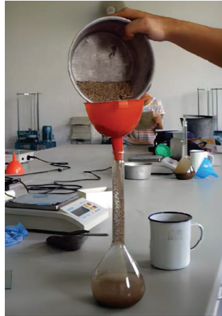
Figure 2. Sand apparent density test.
