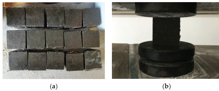
Figure 3. Cube specimen of the compressive strength test and test process. (a) test specimen; (b) test process.
