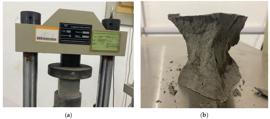
Figure 8. Unconfined compressive strength test: (a) specimen loading process; (b) typical failure mode of the specimen.
