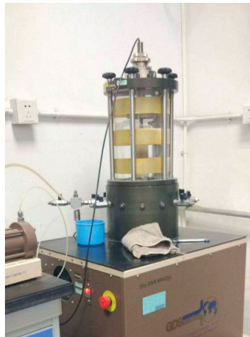
Figure 7. Pressure hood installed.
