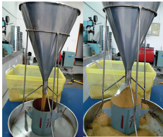
Figure 3. Feeding funnel charging.
