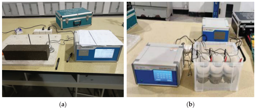
Figure 3. Concrete durability tests. (a) Frost resistance test; (b) RCM test.
