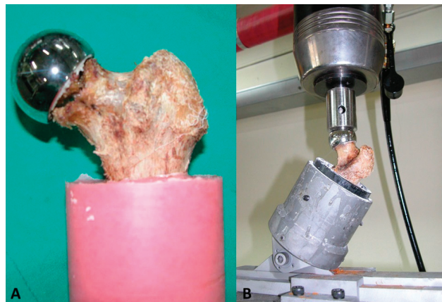
Figure 3. The preparation of the femoral specimens. (A) The femoral specimen was inserted in the resin block along the anatomical axis. (B) The femoral specimen with the femoral head implant was placed in a custom-made jig for the loading–unloading test.
