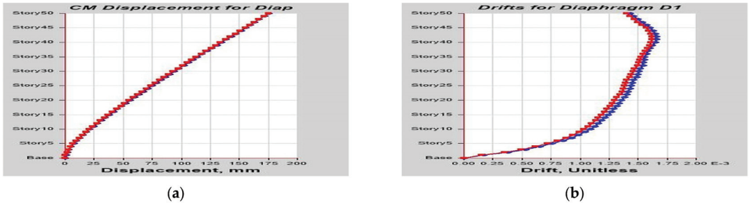
Figure A11. (a) CM Displacement for Diaphragm D1; (b) Drift for Diaphragm D1.
