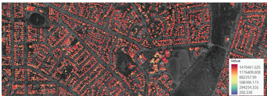
Figure 5. Rooftop solar irradiation potential raster.
