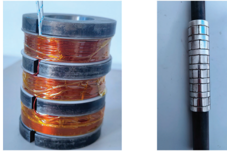
Figure 8. Winding unit and Halbach array of PMLG.
