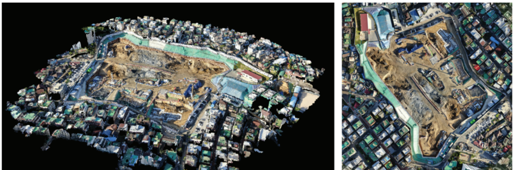
Figure 5. Drone data processing results of 3D point cloud (left) and orthomosaic (right) [70].
