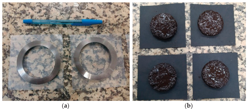
Figure 11. Preparation of microsurfacing asphalt samples for cohesion test: (a) molds used in the test and (b) samples in the curing process.
