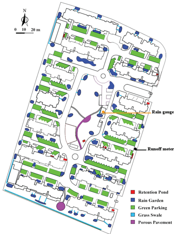
Figure 2. The layout of LID facilities and their combination in the study area.
