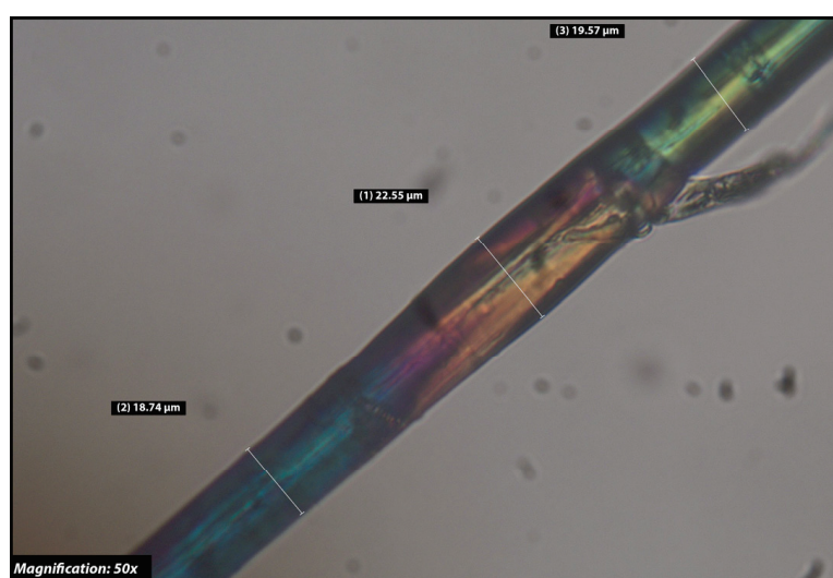
Figure 4. Amorphous and crystalline regions of N-HEMP fibre under the microscope.
