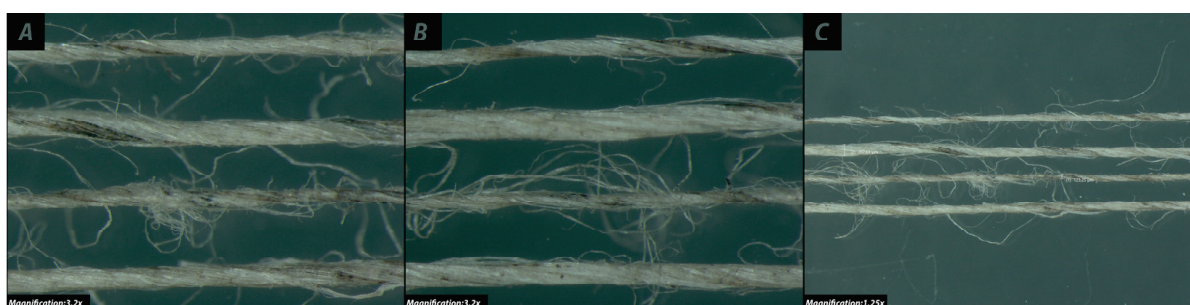
Figure 2. The thickness of N-HEMP under the microscope at different places and magnifications of 3.2 \times (A), 3.2 \times (B) and 1.25 \times (C).
