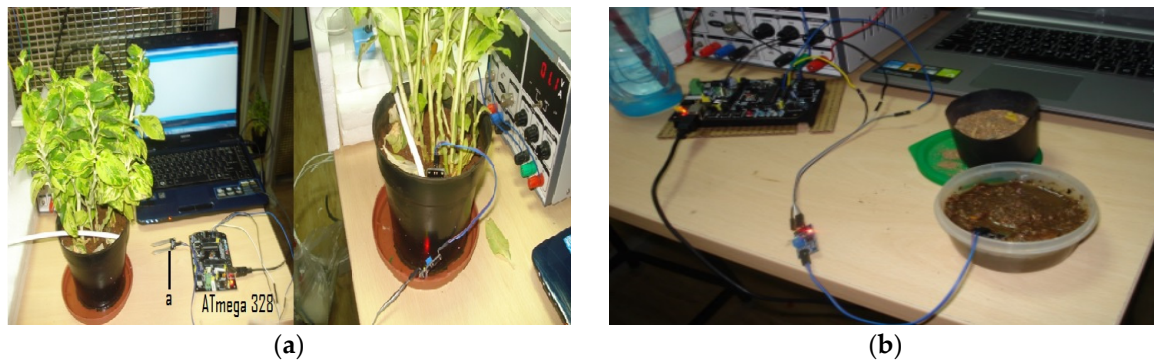
Figure 5. (a) Soil moisture sensor and pH sensor installed and tested; (b) soil moisture sensor placed in panchagavya.
