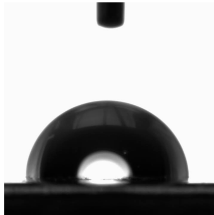
Figure 7. The picture of a water droplet applied on the surface of a MOD4-modified sample.
