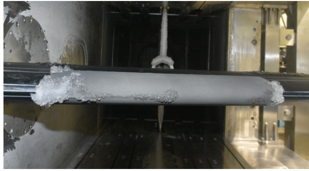
Figure 16. Ice formation on the leading edge at a power density of 4 \text{ kW/m}^2 .
