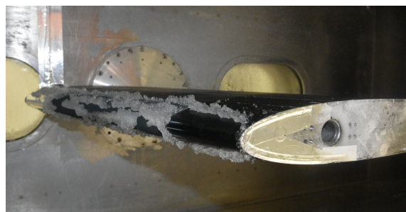
Figure 14. Leading edge ice formation when only sheet A was turned on.
