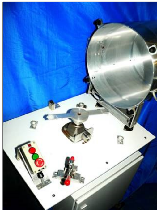
Figure 1. Overview of the centrifuge apparatus. Equipped with an accelerometer, the iced beam is rotated until the ice is detached and captured by the pan.
