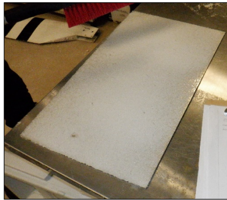
Figure 7. Partially melted and refrozen snow over aluminum reference plate of 30 cm by 50 cm.
