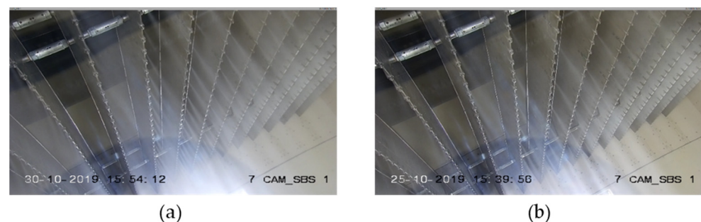
Figure 1. Pattern configurations of spray bar nozzles: 1:2 grid, one half of the spray bar nozzles working (a); 1:4 grid, one quarter of spray bar nozzles working (b).
