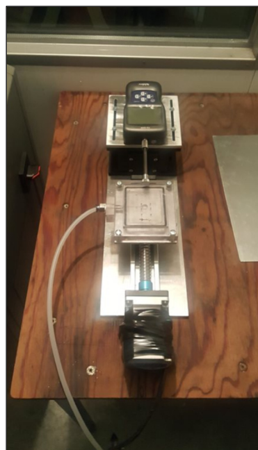
Figure 2. Overview of the push-off apparatus. The ice adhering to the coating is pushed off by the force gauge and evaluates the adhesion.
