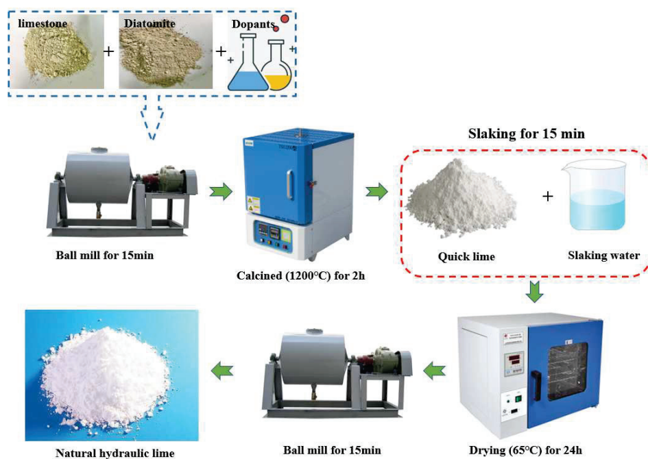
Figure 2. Schematic diagram of preparation process of natural hydraulic lime.
