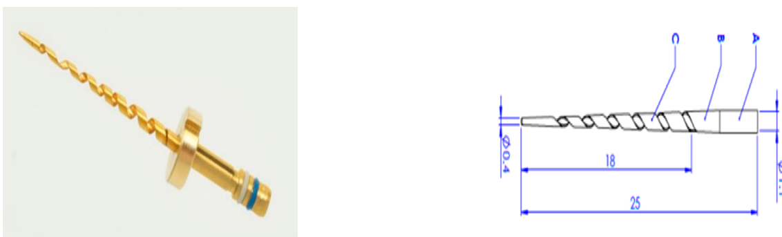
Figure 1. An image of the side-firing spiral Endo tip. The tip is hollow, conical and has a round cross-section with circumferential spiral slits along its entire length. It has three zones: A. the cylindrical sleeve zone (4 mm), which is inserted into the handpiece; B. the flexibility zone (3 mm), which allows additional flexibility when the tip is in action in the root canal; and C. the functional area (18 mm) with six spiral slits. The width of each slit and the distance between them varies so that the width of the furthest apical side slit is narrower (0.4 mm) than the width of the slit located on the coronal side (1.1 mm). The end of the Endo tip is sealed.
