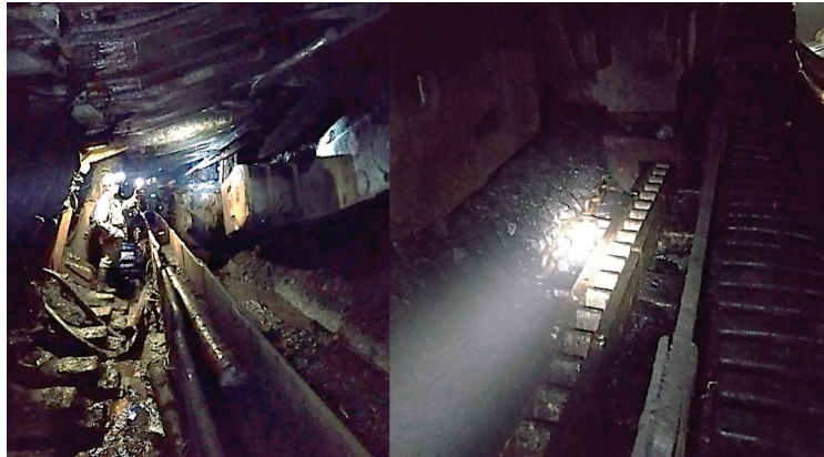
Figure 21. View of the shearer during the underground tests with the Komtrack haulage system in Piast–Ziemowit coal mine.
