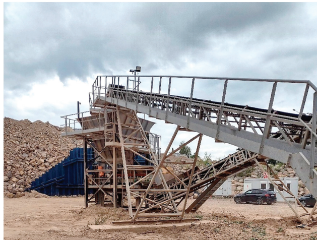
Figure 9. Belt feeder with VSSs (V-type stationary supports).
