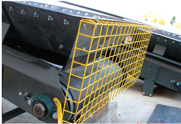
Figure 5. Belt feeder's return pulley with a charging hopper and a safety net.
