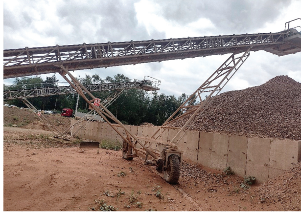
Figure 10. Belt feeder with VMSs (V-type mobile supports).
