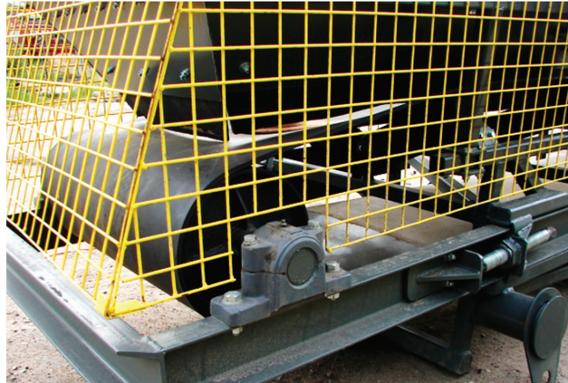
Figure 3. Belt feeder's return pulley with a belt tensioning system.
