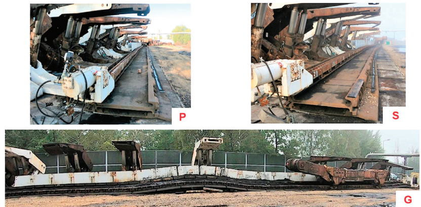
Figure 10. Three alternatives of situating the trough of the armored face conveyor simulating the conditions of underground operation: P—straight route of the conveyor, S—the route of the conveyor deflected in the horizontal plane by 800 mm, G—the route of the conveyor deflected in the vertical plane by about 300 mm.
