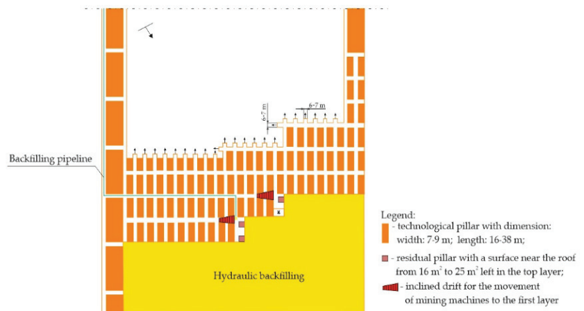
Figure 19. A two-layer room and pillar mining method with a hydraulic backfill in the case of the exploitation gate conditions made of rocks strongly prone to rock bursts.
