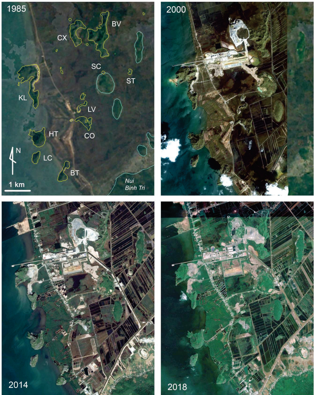
Figure 9. Evolution of limestone quarrying in the MDL-HC karst from 1985 to 2018. Year 1985: before quarrying; abbreviations of hills as in Figure 1A. Photos Google Earth.
