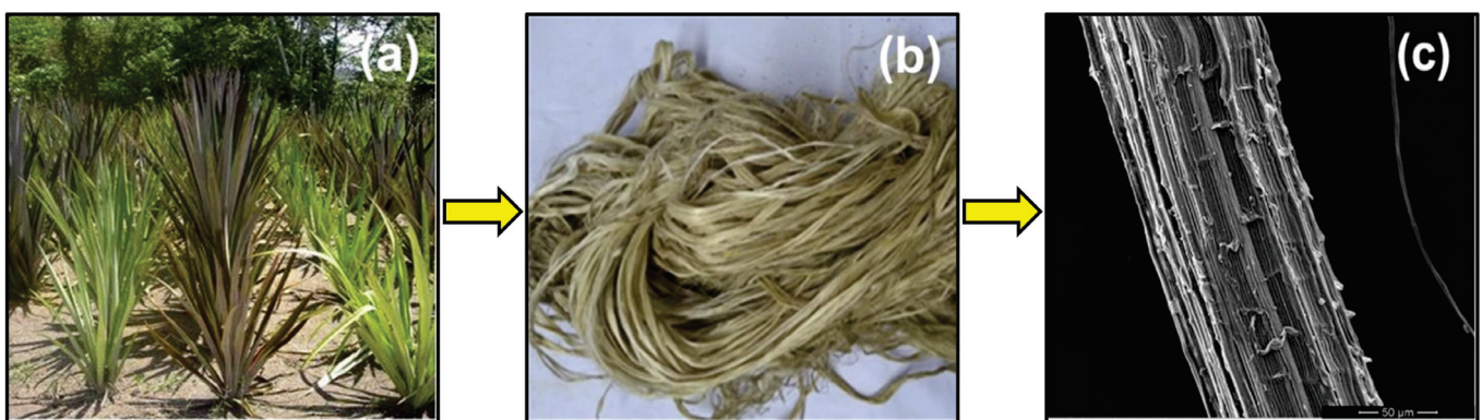
Figure 13. Curauá ( Ananas Erectifolius ): (a) curauá plant; (b) bundle of manually extracted fibers; (c) SEM micrograph of a cross-section of a curauá fiber. Reprinted with permission from ref. [234]. Copyright 2020, Elsevier. Licensed under CC BY-NC-ND 4.0.
