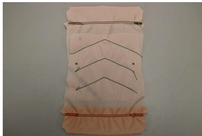
Figure 4. Example of a specimen for testing the seam geometry.
