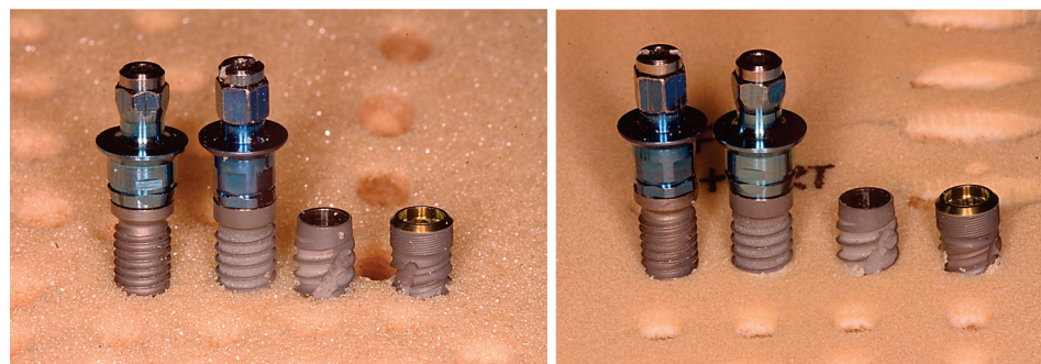
Figure 8. The four implants inserted in the sheets of 10 PCF in density without (on the left) and with (on the right) the cortical sheet.
