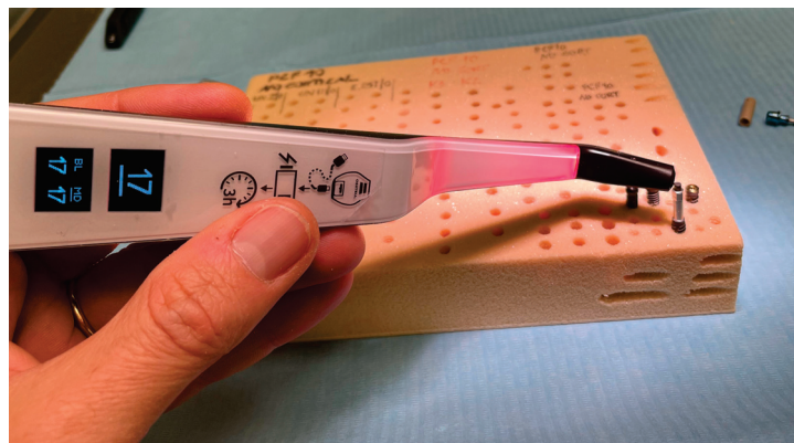
Figure 10. An example of RFA measurements (BL and MD) evaluated on a TAC implant after the insertion in the sheet of 10 PCF in density without the cortical sheet.
