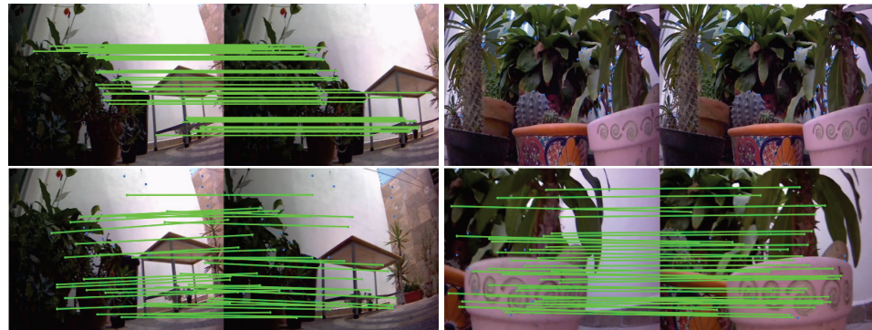
Figure 9. Examples of matched points between key images for Dataset D2. (Top row): ORB+MAGSAC. (Bottom row): LoFTR+MAGSAC.
