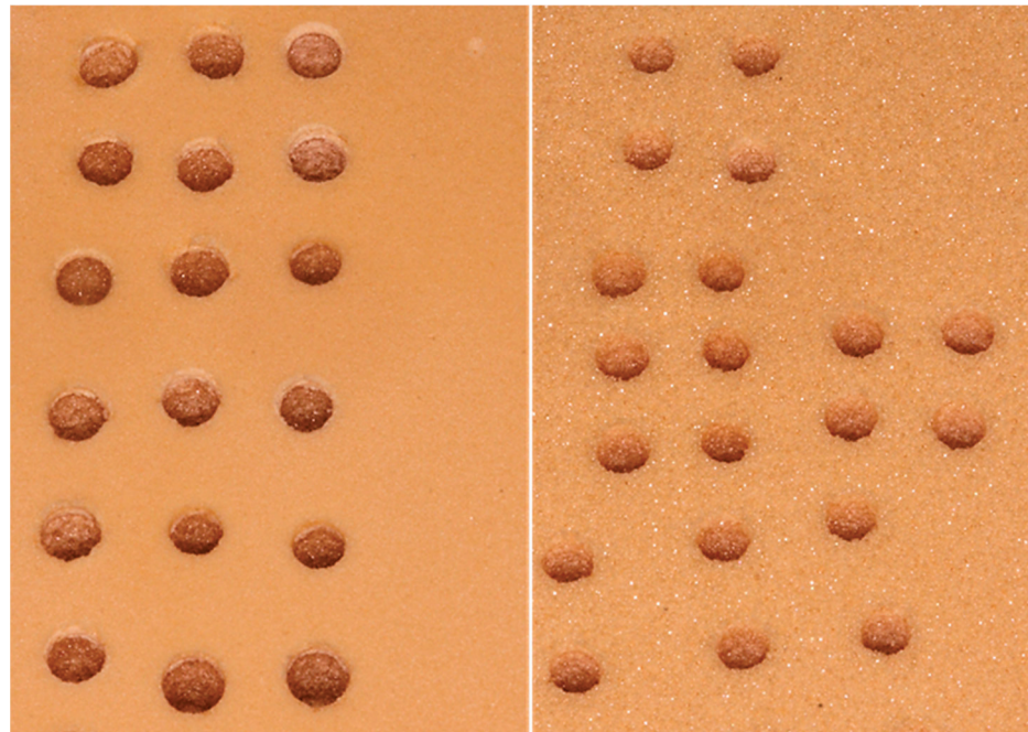
Figure 7. An example of sheets of 20 PCF in density with (on the left) and without (on the right) the cortical sheet of 30 PCF in density.
