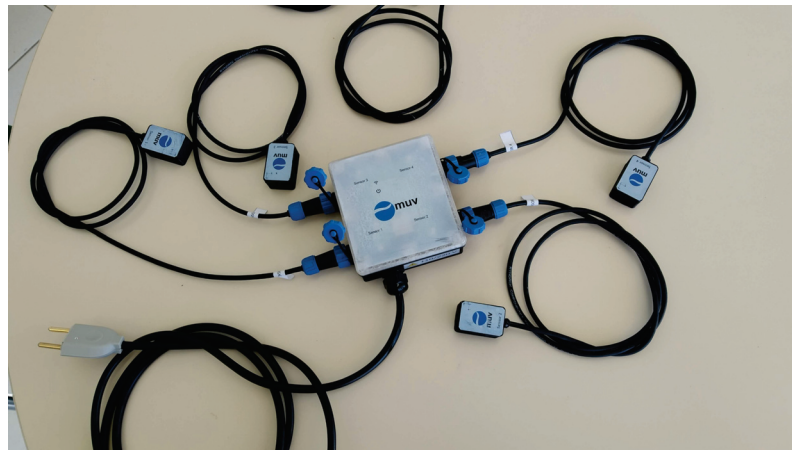
Figure 2. A vibration monitoring system composed of 4 sensors for simultaneously measuring 4 points in the same rotating machine [15].
