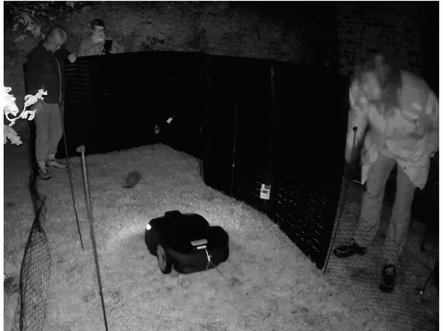
Figure 3. A photo from the surveillance camera used during the encounter tests, illustrating the experimental design. A range of safety precautions for the tests can be seen: (1) a person standing on the right side of the test area stepping in to manually turn off the robotic lawn mower by pushing the (visual) button on the shield of the mower; (2) the rope attached to the back of the mower (with a person pulling it in the other end); and (3) the hedgehog rehabilitator standing inside the test area next to the hedgehog ready to intervene, if necessary. The two persons standing in the vicinity of the hedgehog tested (the hedgehog rehabilitator and the person recording with the handheld FLIR E54 Thermal Imaging camera) remained the same throughout all tests and were cautious to behave in the same manner during all tests.
