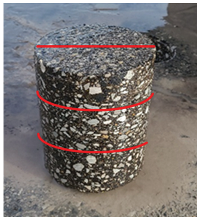
Figure 1. Cuts made along the red lines to prepare a semicircular specimen with a thickness of 50 mm.
