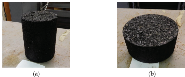
Figure 1. Compacted 100% RAP emulsified cold mix specimens: (a) Proctor and (b) SGC.
