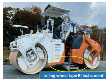
Figure 1. Vibratory roller with rolling wheel-type RI instrument.
