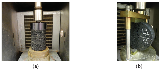
Figure 2. Specimen setup for (a) compression test and (b) indirect tension test.
