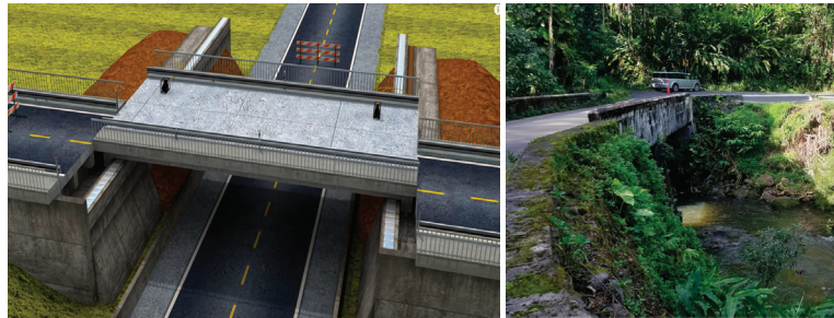
Figure 3. General schematic of the lateral bridge slide technique, and a view of the typical site conditions around the structures. (Source: https://www.youtube.com/watch?v=YzYCSw5mACQ , accessed on 7 July 2023, FHWA—CFLHD).
