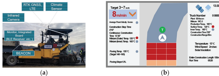
Figure 2. IoT PQMS related to asphalt paver: (a) Installed sensor; (b) Monitor.
