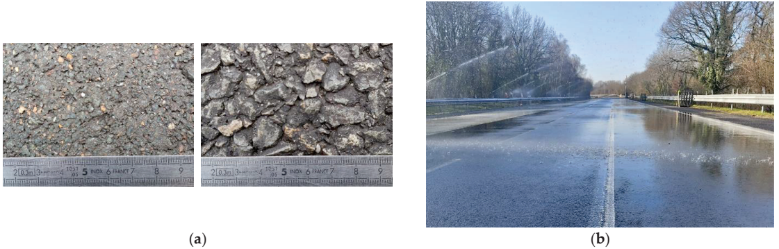
Figure 3. Test tracks: (a) test surfaces; (b) wetting system.
