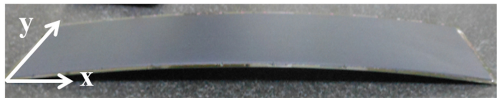
Figure 3. Actual strip warpage on the production line.
