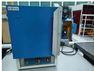
Figure 2. Heat treat furnace.
