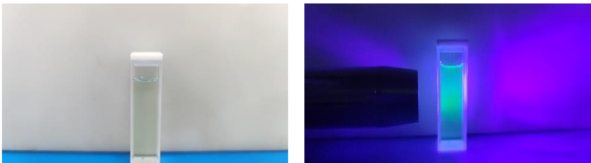
Figure 5. Color development of CQD-W under natural light (left) and UV light (right) irradiation.
