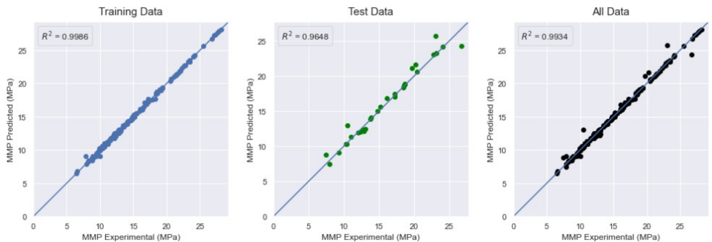
Figure 24. Plot of predicted versus experimental values of minimum miscibility pressure.
