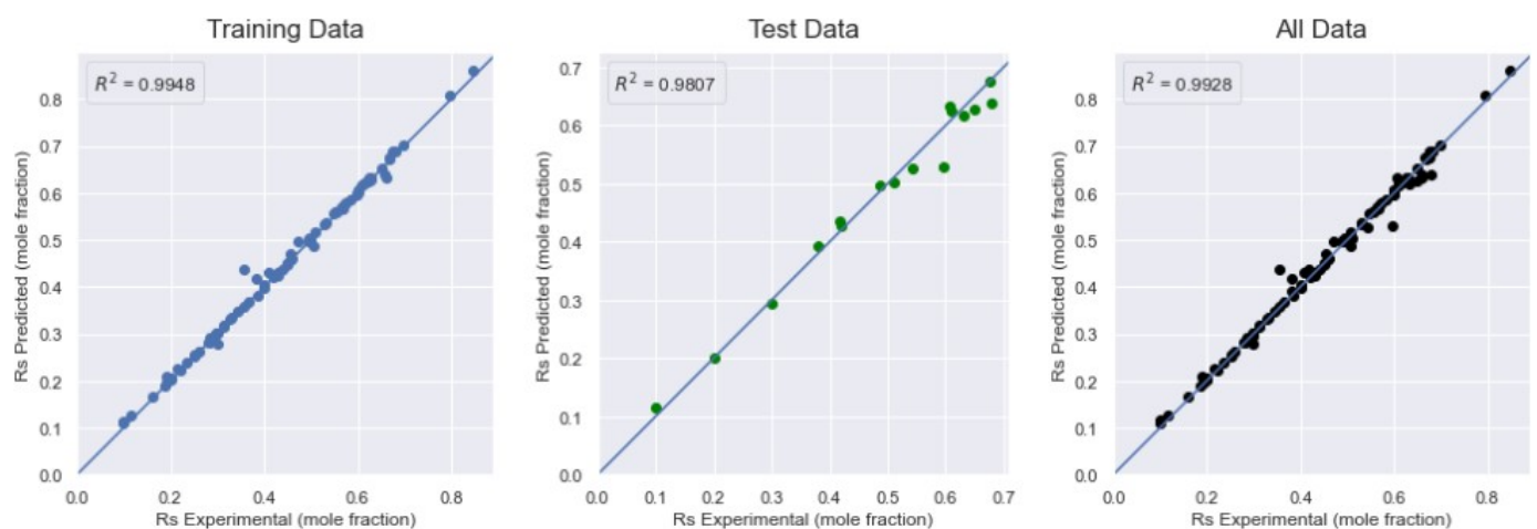
Figure 14. Comparative plot of predicted and experimental dead solubility values: an analysis of training data, test data, and the complete dataset.
