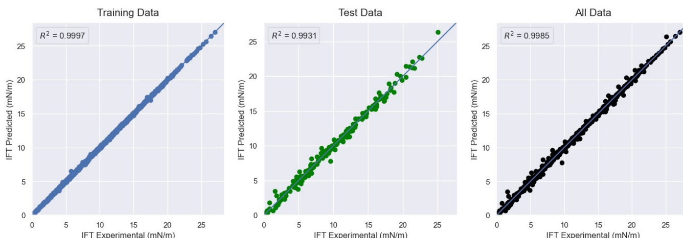
Figure 20. Plot of predicted versus experimental values of interfacial tension.
