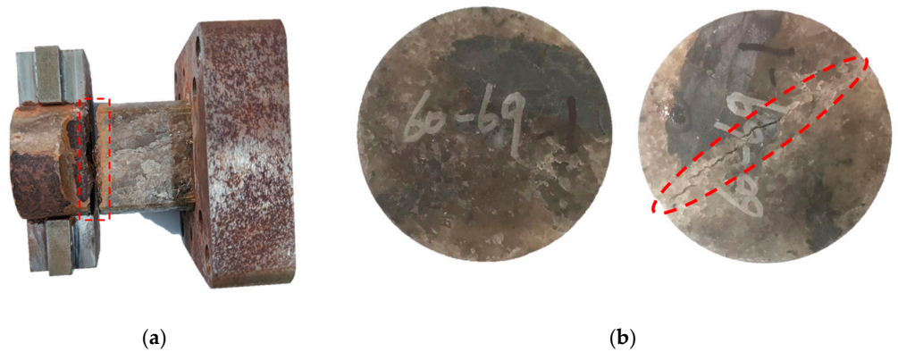
Figure 3. Tensile test photos of salt rock. (a) #5 direct tension (b) #1 indirect tension (left Before experiment, right after experiment).
