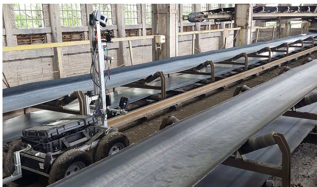
Figure 7. View of the robot during inspection.
