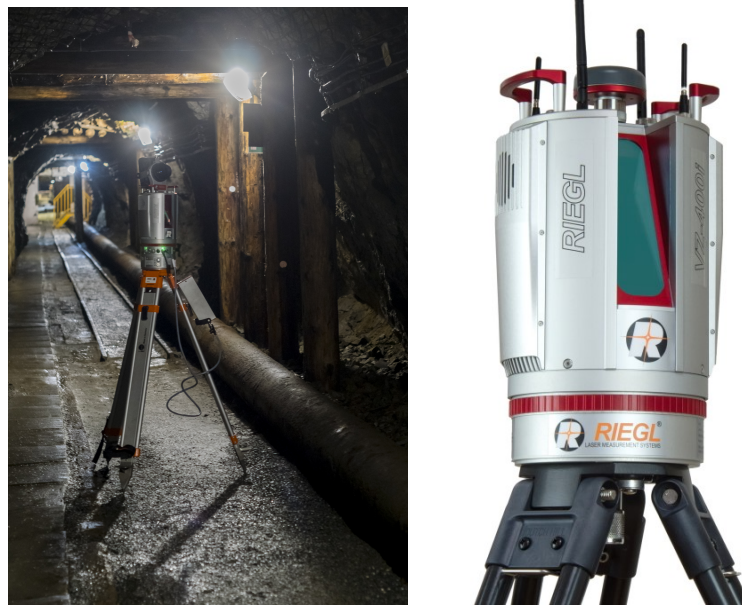
Figure 3. RIEGL VZ-400i Terrestrial Laser Scanner in the adit.
