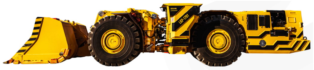
Figure 1. The LHD vehicle under investigation: LKP-1701 (KGHM ZANAM) with a powerful diesel engine for the underground mines [29].
