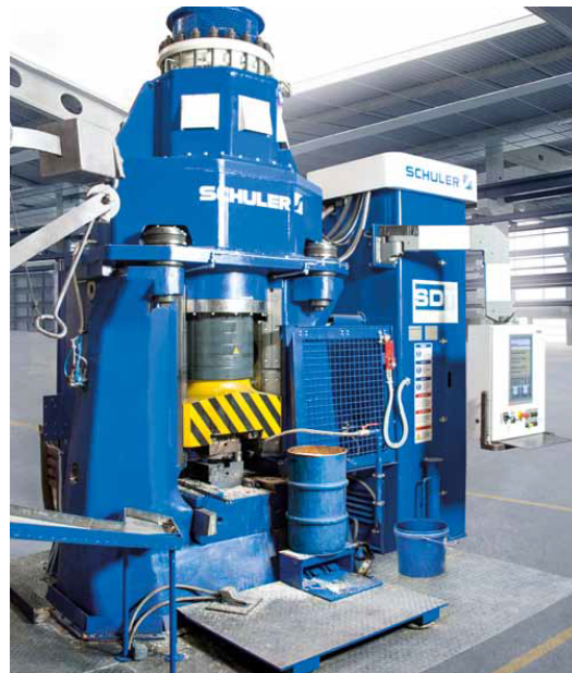
Figure 9. New linear electric forging hammer (Schuler [61]).
