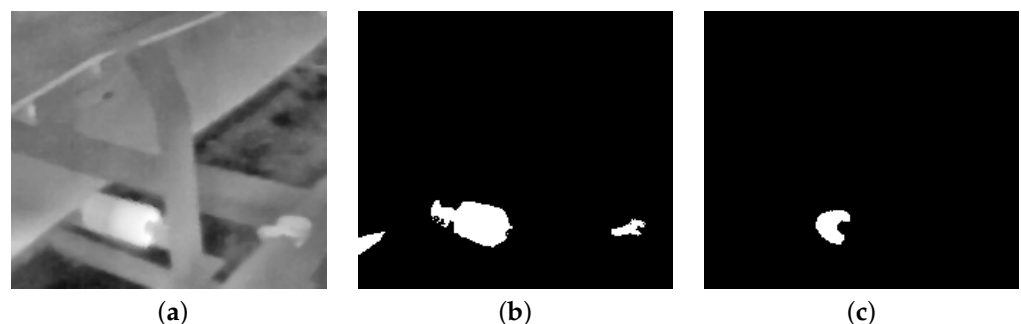
Figure 5. Comparison of extreme and mild outliers in segmentation of an overheated idlers. (a) Pre-processed ROI before segmentation, (b) Segmentation results of mild outliers detection, (c) Segmentation results of extreme outliers detection.
