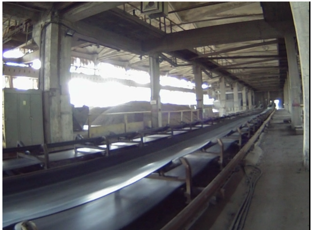
Figure 8. A general picture of the raw materials storage with belt conveyor to transport raw materials.
