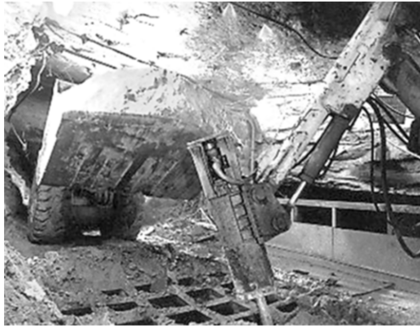
Figure 11. The dumping point with a screen and hydraulic hammer on the manipulator in the underground mine (Stefaniak et al. [87]).
