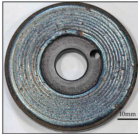
Figure 3. Fe 3 Al coating with Ferro 55 buffer layer deposited on GCI substrate.
