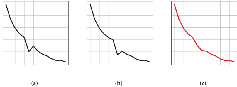
Figure 1. Examples of similar subsequences (a,b) and the average subsequence of these subsequences (c).
