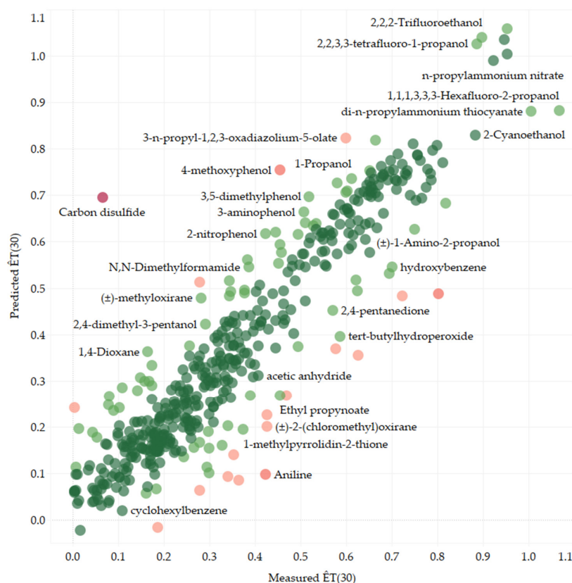
Figure 1. Experimental vs. Model 3-predicted \hat{E}_T(30) values for 461 solvents colored by absolute error.
